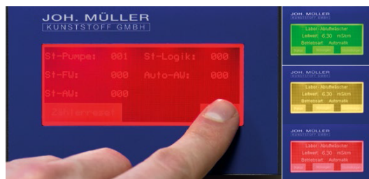
Interactive touch display for operation and status information (green/yellow/red).
