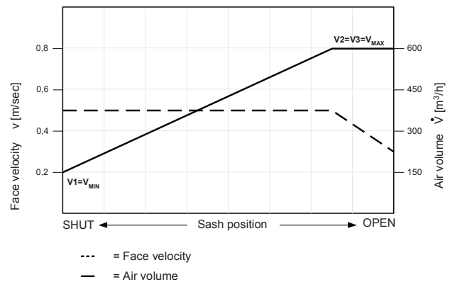
Figure 2: Linear sash position control
